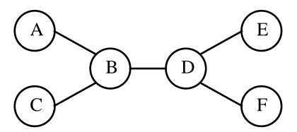
Theorem: if the constraint graph has no loops, the CSP can be solved in  $O(n d^2)$  time
