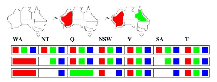
NT and SA cannot both be blue! Constraint propagation repeatedly enforces constraints locally
