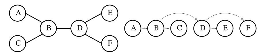
2. For j from n down to 2, apply Make-Arc-Consistent  $(Parent(X_j), X_j)$  (will remove inconsistent values)
