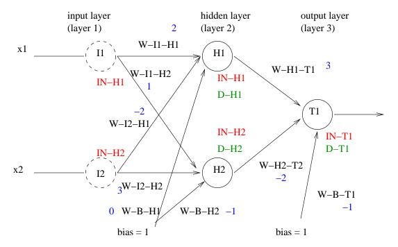
Each neuron is connected to all the neurons in the next layer, there are no back connections (this is a *feedforward network*).
