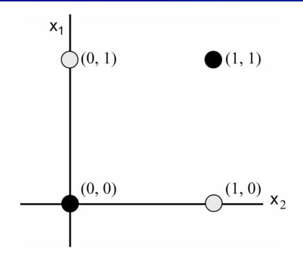
No straight line in two-dimensions can separate the (0, 1) and (1, 0) data points from (0, 0) and (1, 1).
