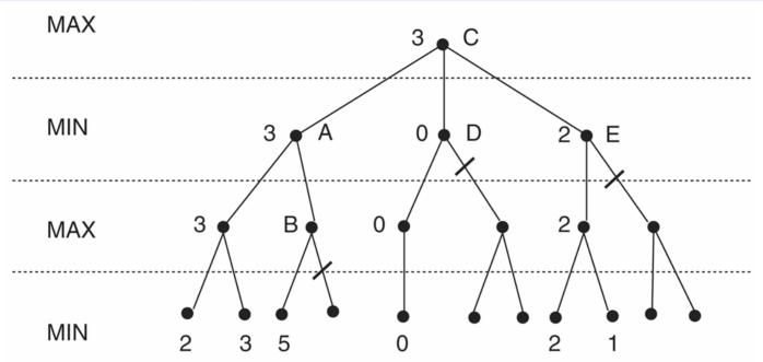
A has  $\beta = 3$  (A will be no larger than 3) B is  $\beta$  pruned, since 5 > 3C has  $\alpha = 3$  (C will be no smaller than 3) D is  $\alpha$  pruned, since 0 < 3E is  $\alpha$  pruned, since 2 < 3C is 3 Pruning does not affect final result
